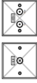
Old isolated outlet plates - not compatible with proSAT1EYE
