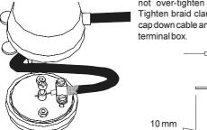
not over-tighten terminal screw. Tighten braid clamp screws, ease cap down cable and fit securely onto
